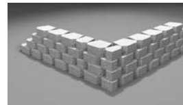
Alternate orientation of corner half units with each subsequent course.
