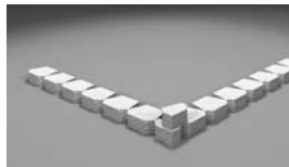
Start outside corner with a half unit.
