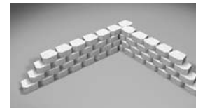
Use full blocks in the corner of inside corners.
