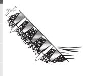
\*A slope of 1 in 1 is possible if every block has suitable anchoring in one of the cores into the subsoil and the site has been assessed to ensure global
